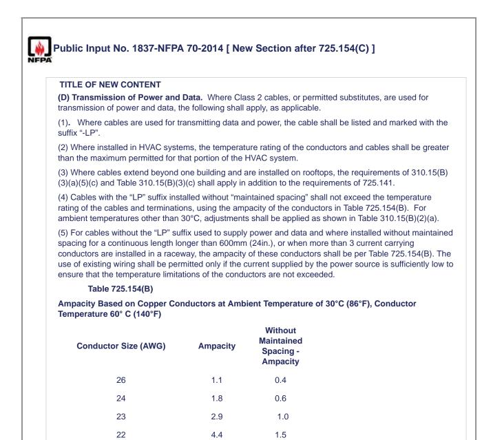
Informational Note: Table 725.154(B) shows the current permitted in each conductor of a multi-pair cable.
