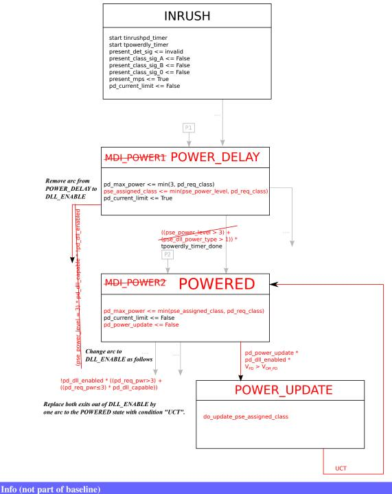
The following non-normative text is added to explain that it is not permitted to draw more power than the requested Class. The actual requirement is in the PD state diagram, as well as on D2.2, page 153, line 47.
