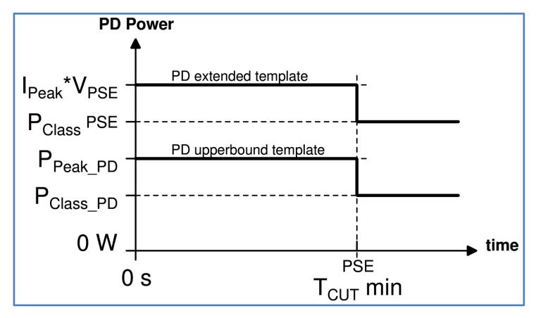
Info: The extended template is based on PSE PI parameters. At Rchan = Rch the extended and upperbound template lines are fully overlapping.
