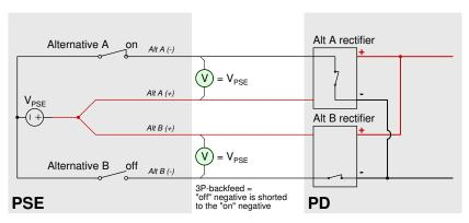
Just like the PSE shorts the positive pairs together, the some PDs short the negative pairs together when exposed to 3-pair power ( $2 \times positive$  and  $1 \times negative$  voltage).
