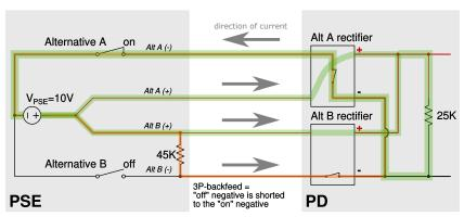
If the PSE ties an "off" negative pair to the positive and the PD connects the negative pairs together, this causes the PSE discharge resistor to appear in parallel to the PD detection resistor.  $\Rightarrow$  PDs may not tie negatives together in the detection voltage range.
