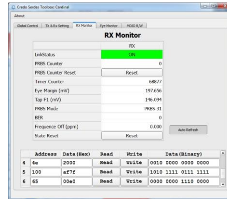
2m no-FEC link enabled by Credo 50Gb/s NRZ PMD
