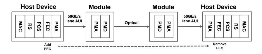
Then the worst case input BER for the FEC decoder must be met by the concatenation of all of the sub-links.
