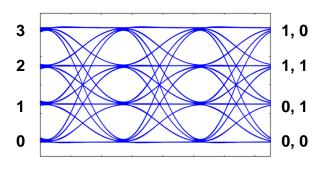
Since two of the eight possibilities result in both bits being correct, these states terminate the burst. Therefore for Gray coded PAM4, if a **symbol** is in error, the worst case probability that the next **symbol** is also in error is 0.75.
