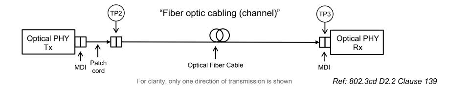
In current IEEE 802.3 PHY's the optical link between transmitter and receiver, i.e. between TP2 and TP3, is in the form of a passive connection over a fiber optic cabling (channel).
