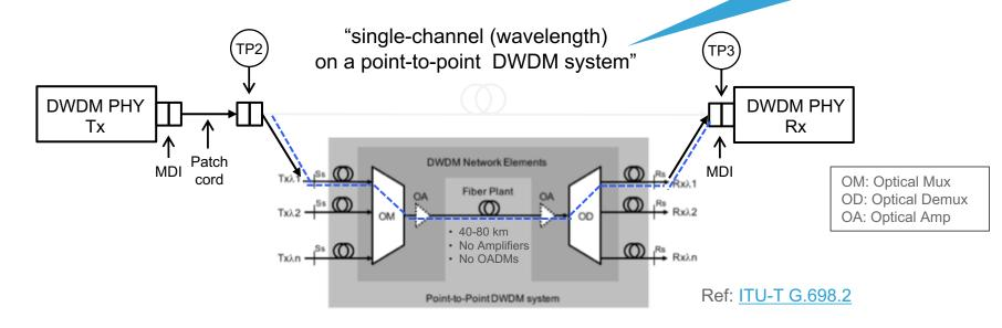
In this example the "DWDM PHY" runs over an optical channel comprising of  $\lambda$ 1ports on the point-to-point DWDM system, using the 'black link' approach from ITU G.698.2
