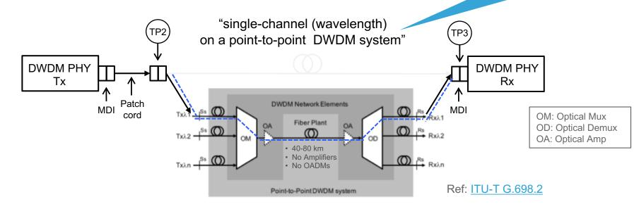
As in the case of the traditional Ethernet optical PHY the optical reference channel (shown above) will be **used** to help define the optical interface parameters at TP2 and TP3.
