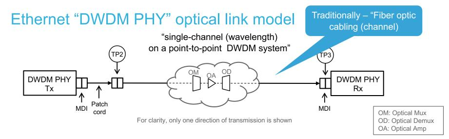
We need to define a "DWDM PHY" where the optical link between transmitter and receiver, i.e. between TP2 and TP3, is in the form of an optical channel connected over single-channel (wavelength) ports of a point-to-point DWDM system (optical mux, optical amplifier, fiber, optical demux).
