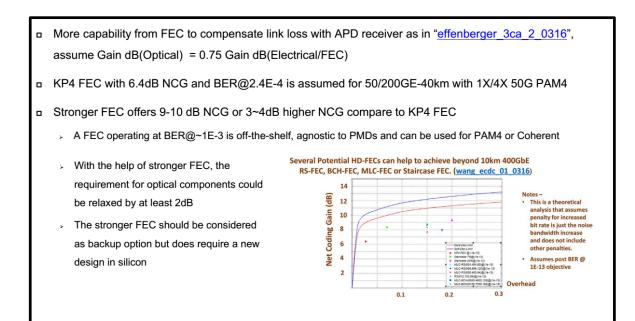
In yamamoto\_b10k\_01a\_0118, high data rate test result to support more optical margin and available of stronger FEC based on generic RS FEC.
