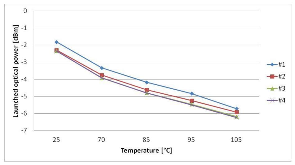
Graph above shows the average LOP of 4 samples across temperature. 16-PAM baseband modulation was used for the measurements.
