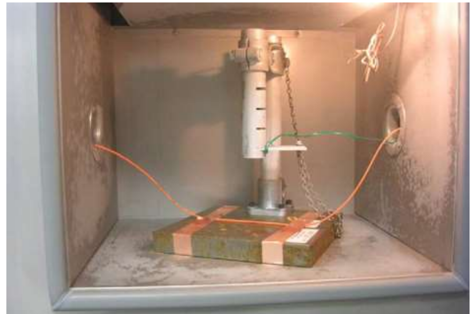
Impact test setup at -20C
