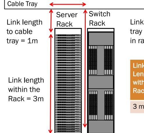
Link length from cable tray to any switch port in rack Switch = 4m
