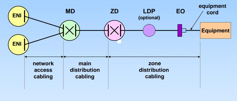
ENI = Equipment Network Interface MD = Main Distributor ZD = Zone Distributor LDP = Local Distribution Point EO = Equipment Outlet
