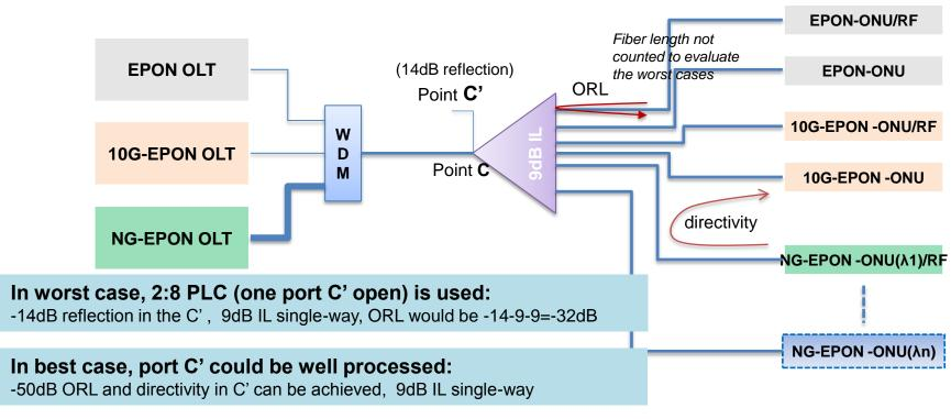
It was found that particularly many 1:8 splitter were in fact made by 2:8 PLC chips (that means the splitter is really a 2:8 splitter with one port open in the package box).
