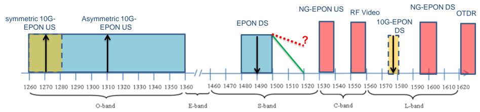
In case of NG-EPON coexisting with EPON, the guard band from upper edge of EPON downstream (1500nm) to lower edge of NG-EPON upstream band (1530nm) is 30nm.
