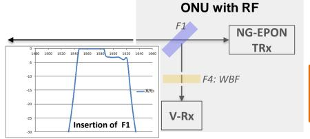
Assuming **S** represents the V-Rx sensitivity at -12dBm **Reflected interference signal is defined by X**
