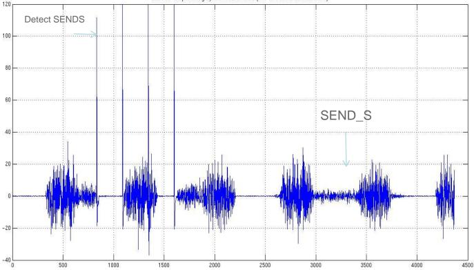
Slave MF output during Synchronization state ( PN-255 with 0 dB burst noise)
