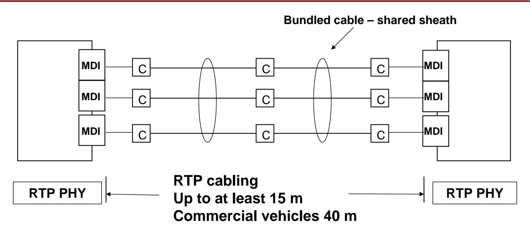
RTP Link transmission and coupling parameters
