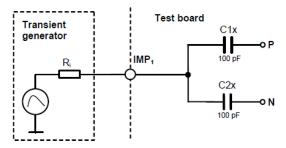
The measurement of immunity against transient pulses shall be tested using the capacitive coupling clamp according to ISO 7637-3: 2007-07 (CCC method) and using the current probe (BCI) according to ISO 7637-3: 2007-07 (ICC method).
