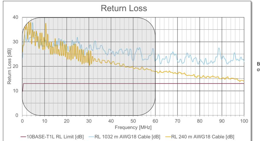
Below 32 MHz the frequency resolution of the VNA is 125 kHz, above 250 kHz.
