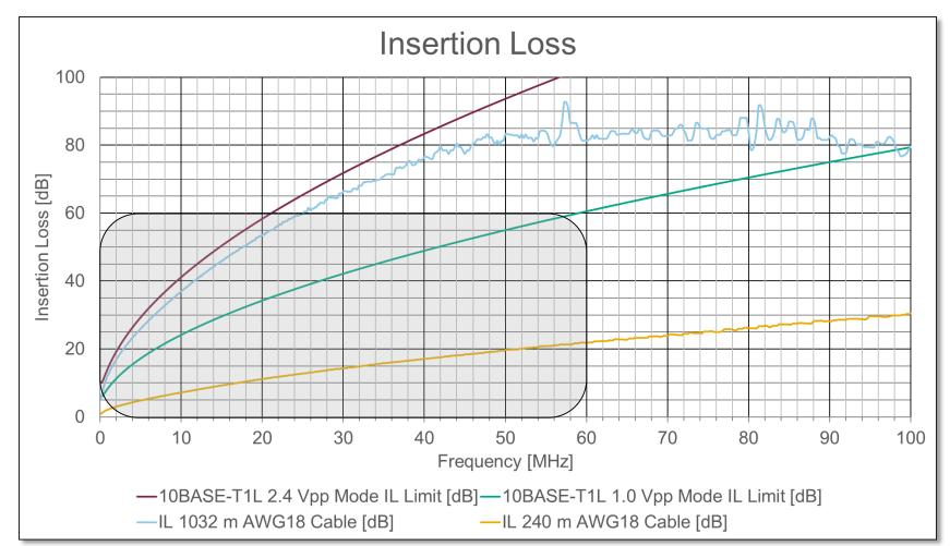
• Measuring Fieldbus Type A cables suitable for 10BASE-T1L; also at higher frequencies the cables behave pretty well, above 30 MHz it seems that some small structural return loss is visible in the measurements.
