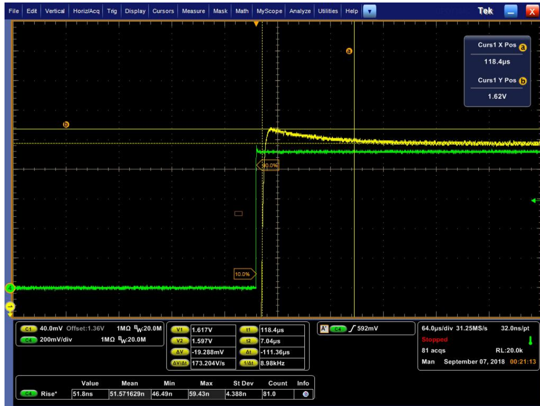
Figure 1-1, 20 channels burst on at same time, -13dBm Per Ch, Monitor one of all channels, Gain excursion:0.5dB
