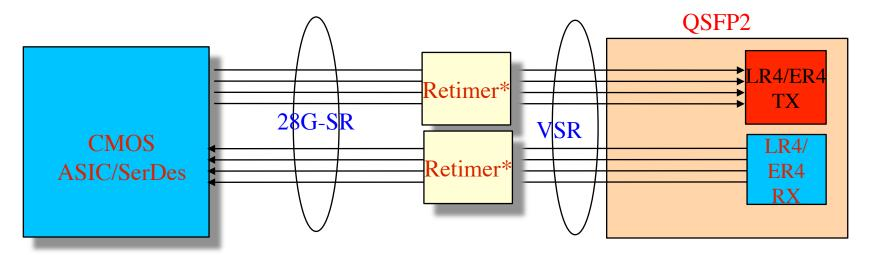
\*Assuming in the case of QSFP2 the retimers are external it solves the power issue and distance
