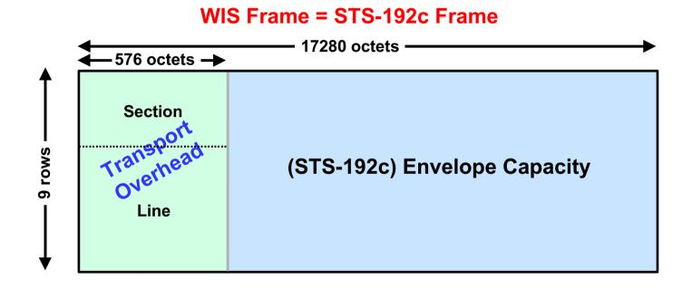
STS-192c = Synchronous Transport Signal – level 192, c = concatenated.
