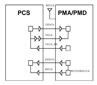
PMA Interface for Serial Transmission
