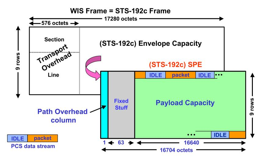
STS-192c = Synchronous Transport Signal – level 192, c = concatenated SPE = Synchronous Payload Envelope
