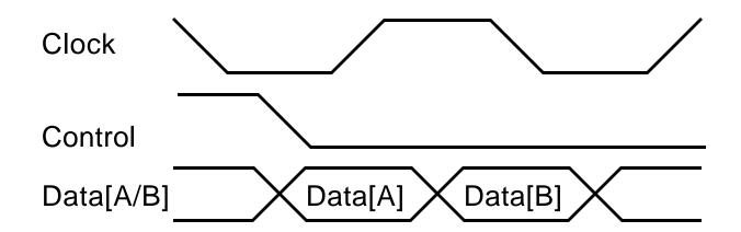
■ 32 bit data paths are divided into four 8 bit "lanes", with one control bit for each lane
