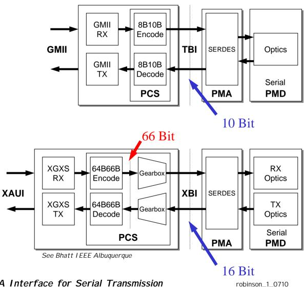
PMA Interface for Serial Transmission
