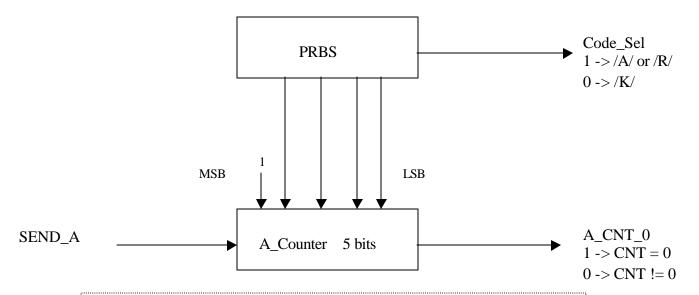
The A\_Counter counts down to zero and is parallel loaded with a random 4-bit pattern from four of the PRBS stages. The MSB is always loaded with a 1 to give the random count between /A/ codes of 16 to 31. It is loaded by the SM when an /A/ code is sent and signals a zero count back to the SM.
