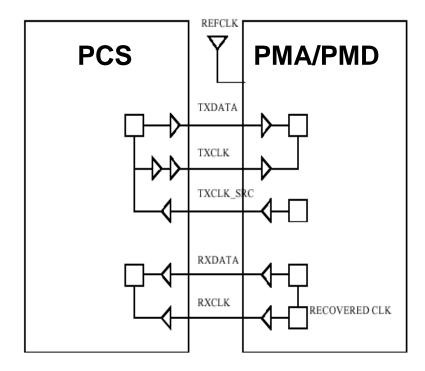
PMA Interface for Serial Transmission
