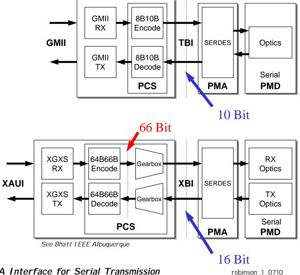
PMA Interface for Serial Transmission
