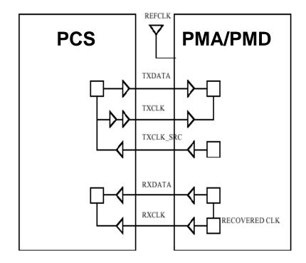
PMA Interface for Serial Transmission
