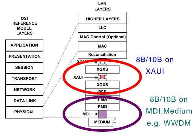
MDI = Medium Dependent Interface XGMII = 10 Gigabit Media Independent Interface XAUI = 10 Gigabit Attachment Unit Interface PCS = Physical Coding Sublayer XGXS = XGMII Extender Sublayer PMA = Physical Medium Attachment PHY = Physical Layer Device PMD = Physical Medium Dependent
