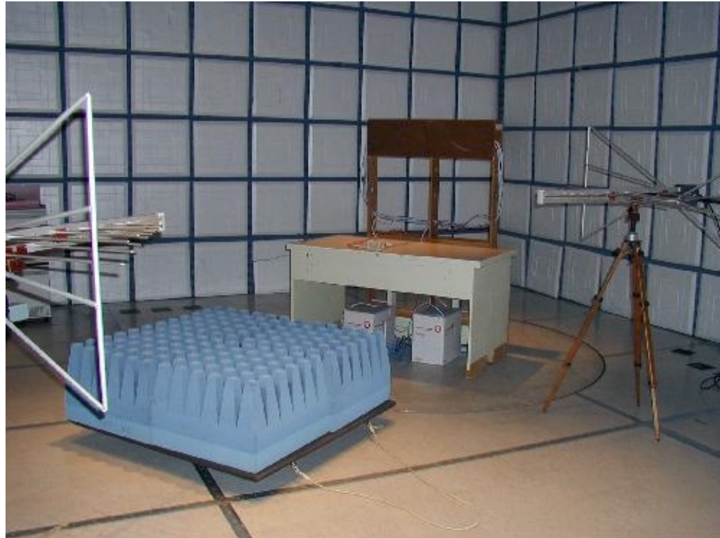
Radiated Susceptibility Test Configuration
