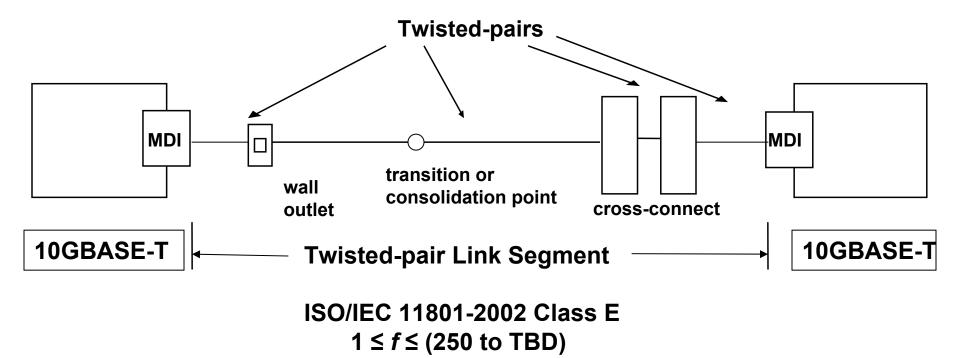
\*Class E Specified:  $1 \le f \le 250$  MHz Class E: 250 < f  $\le$  TBD – starting point for extrapolated frequency performance
