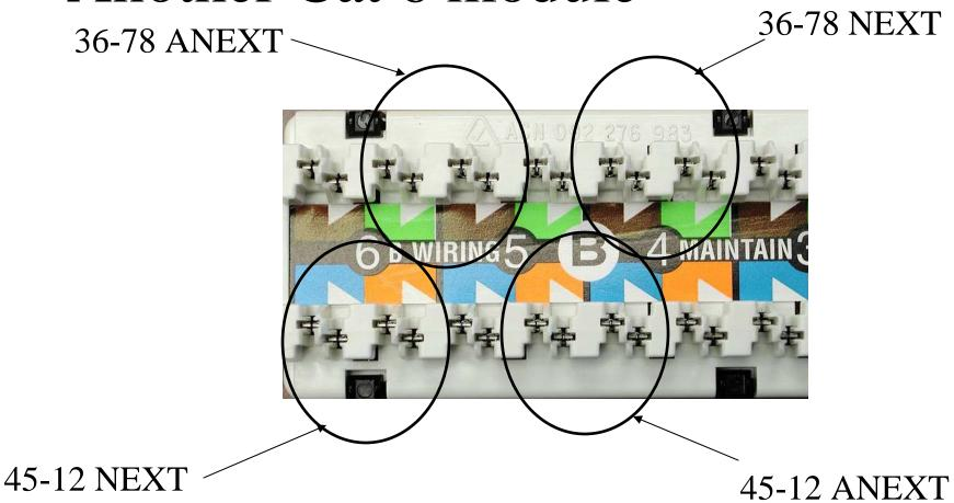
• The 45-12 ANEXT and 45-12 NEXT coupling from IDC occur both internal and external to port. Similar for 36-78
