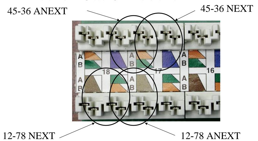
• The 12-78 ANEXT and 12-78 NEXT coupling from IDC occur both internal and external to port. Similar for 45-36
