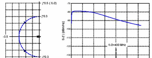
Achievable SNR vs. cable length does not critically depend on exact shape of S<sub>r</sub>(f)
