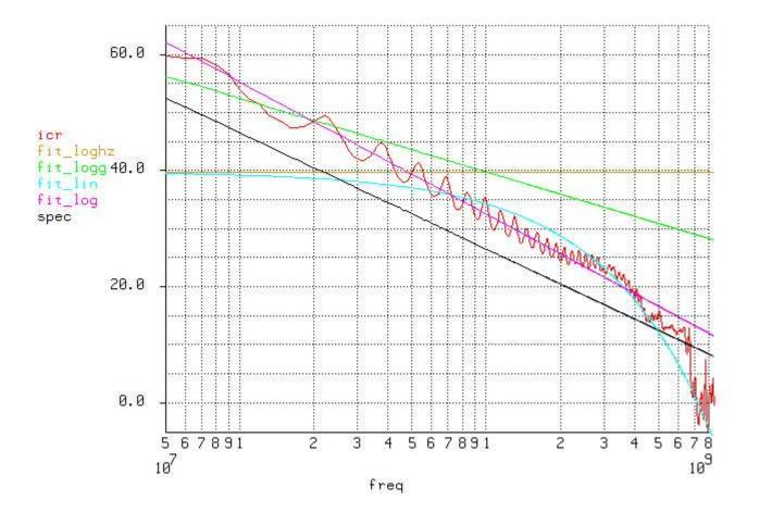
On these plots: The Red curve is ICR The Brownish curve is a literal following of the D'Ambrosia equations. The Green Curve is the D'Ambrosia equations assuming frequency is in GHz rather than Hz The Light Blue curve is a linear frequency fit The Magenta curve is a log fit using equations given below The Black curve is the ICR spec.
