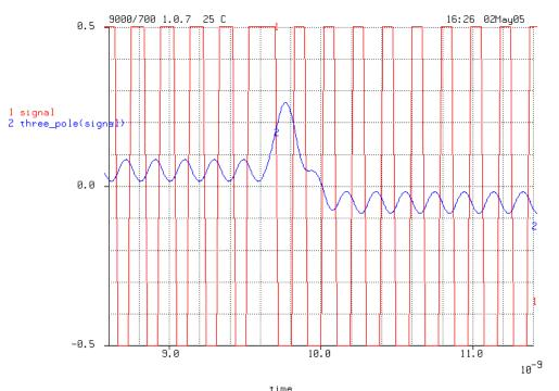
This is an alternating 1010 pattern with 5% DCD before (red) and after (blue) a 10GHz low pass filter with a change in phase so that the even bits are initially 1s, then 0s.
