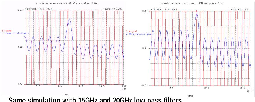
Same simulation with 15GHz and 20GHz low pass filters.
