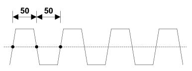
Duty Cycle Distortion (DCD) is both the variance in timing away from 50% duty cycle, and also the variance in average voltage offset.
