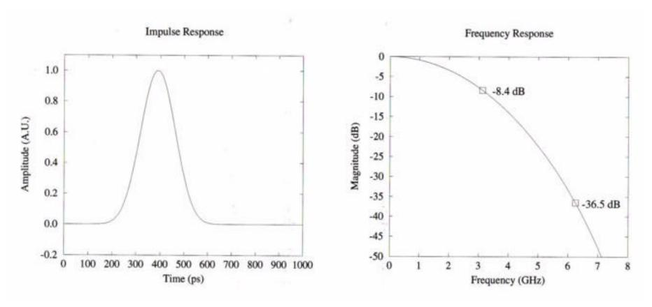
Loss in this example is 28dB greater at 6.25 GHz than at 3.125 GHz.
