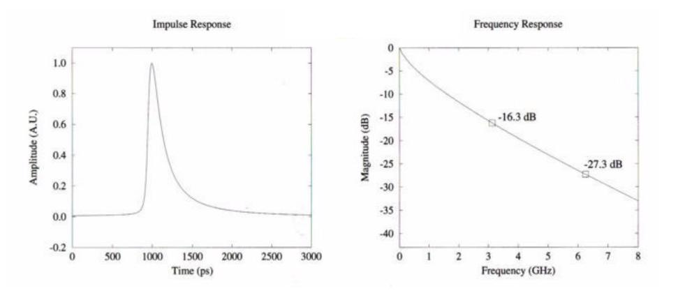
Loss in this example is 11dB greater at 6.25 GHz than at 3.125 GHz. (Should be a candidate for PAM-4.)
