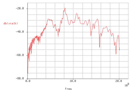
This is the frequency domain version of the NEXT channel associated with Channel A.
