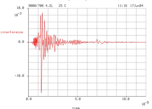
simulation of LP filtered pulse response of UXPi channel A Xtalk
