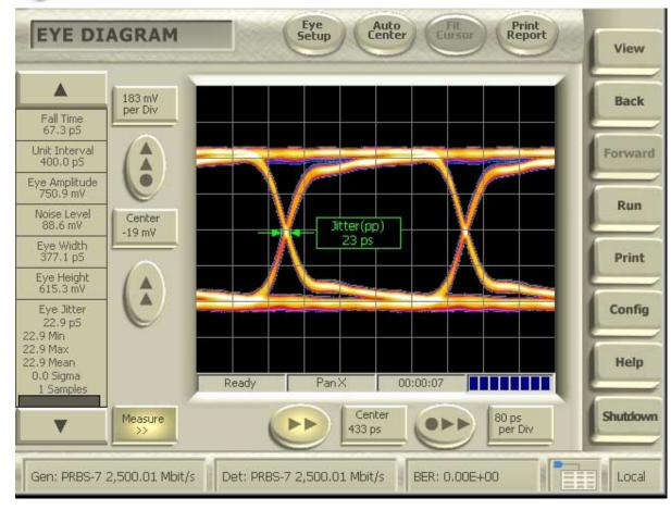
Comparable to sampling scope eye diagram results (rise/fall etc.)
