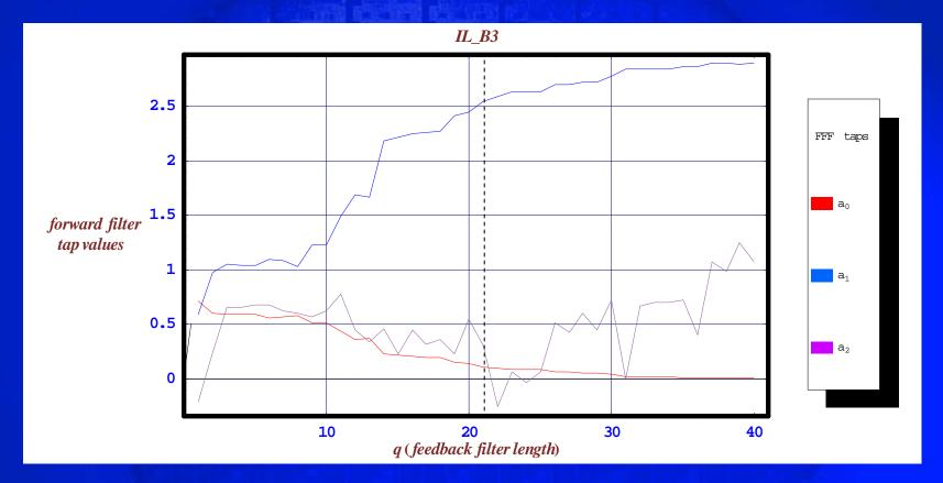
Except for a relatively narrow range, the three taps in the receiver FFE are always providing additional equalization.
