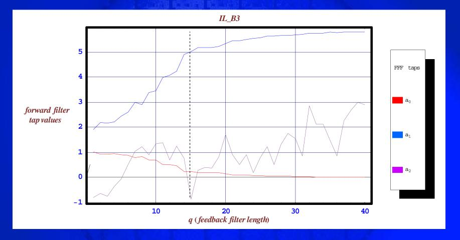
Regardless of the feedback filter length, q, the forward filter is always providing additional equalization. This is consistent with the fact that the NRZ target spectrum differs significantly from the *native* backplane response.
