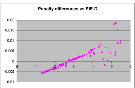
Within 0.02 dB; negative differences possibly explained by round-off errors in PIE-D, simulated waveform, or elsewhere.
