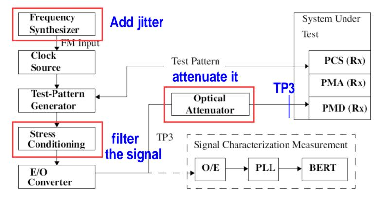
Figure 53–10-Receive jitter test block diagram
