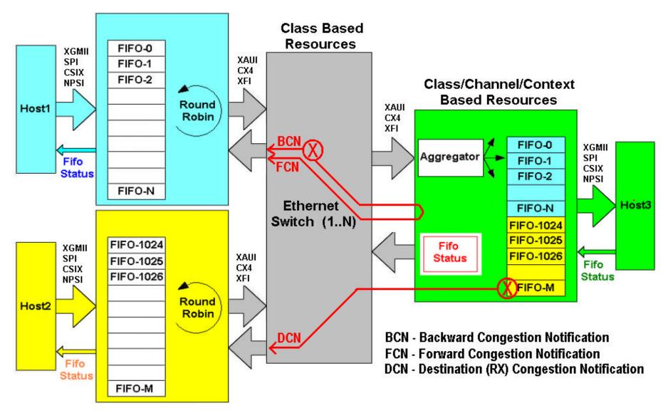
Note: Link-Layer Flow Control provided by "Class" based 802.3x message
