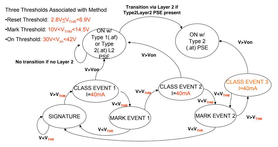
Class Event 3 exists to create a defined behavior for Type 2(.at) PDs when pinged repeatedly. This allows future expansion of the classification mechanism with a known response from Type 2(.at) PDs. PD transitions through Class Event 3 during power on.
