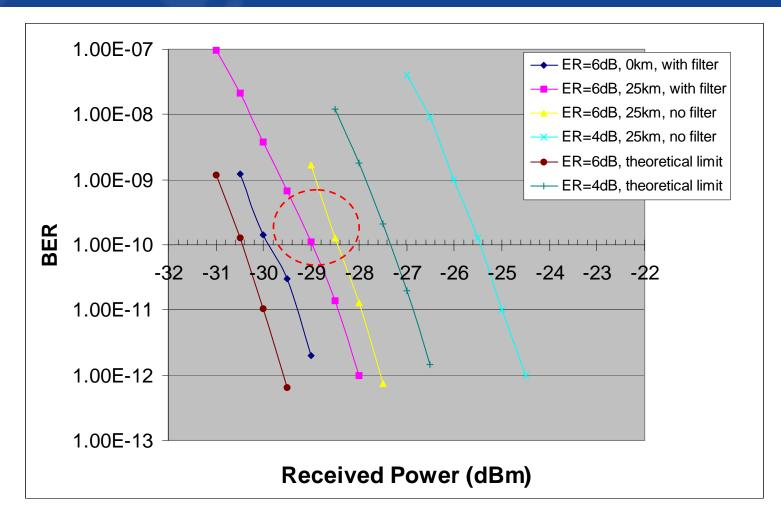
Working at 1535nm avoid need for optical filter Practical sensitivity is -28 dBm
