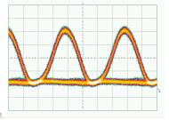
10 Gb/s RZ signal at 6.0 dB into saturation
