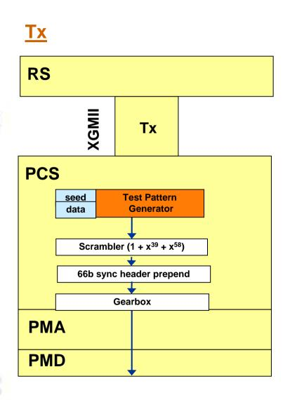
The test patterns are generated by utilizing the regular scrambler and framing mechanisms of 10G:
