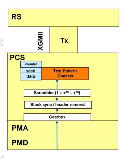
The test pattern data is received by the <u>Checker</u> function via the regular synchronization, framing, and scrambler mechanisms of Serial 10G:
