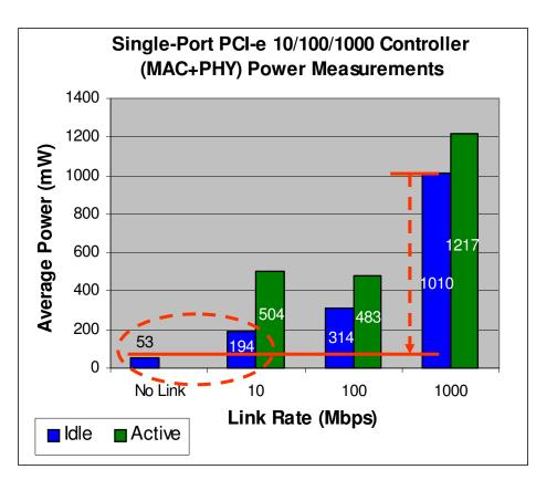
Source: Intel labs. Intel® 82573L Gigabit Ethernet Controller, 0.13µm, "Idle" = no traffic, "Active" = line-rate, bi-directional
