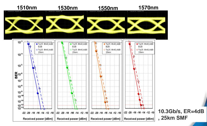
1550nm band CWDM DML is feasible for SMF 10km. Similar result is expected with 1310nm band CWDM DML.
