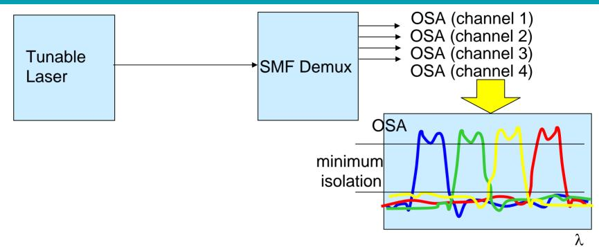
Tunable laser + OSA readout optical isolation measurement
