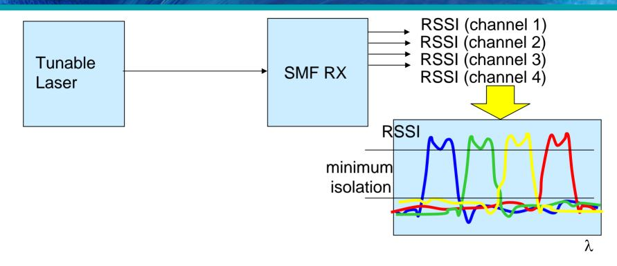
Tunable laser + module RSSI readout optical isolation measurement
