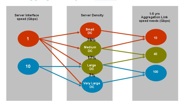
Different classes of Data Centers have different needs (and cost sensitivity) in terms of aggregation link speed.
