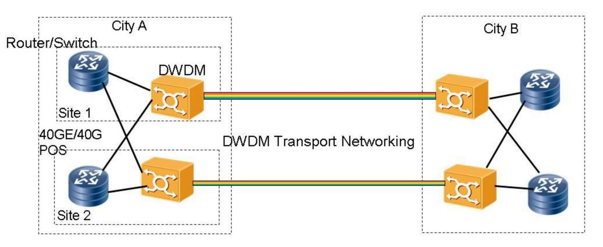
Due to service protection, Routers connection to DWDM equipments with dual-homing configuration
