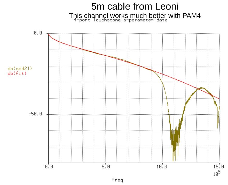
11/09/11 Note: This data is from measurements of 802 3ba compliant QSFP cable assemblies for the purpose of establishing baseline noise impairments beyond those currently specified in 802.3ba, and not for consideration as channels for 25 Gb/s.
