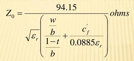
$$c_{f}' = \frac{0.0885\varepsilon_{r}}{\pi} \left\{ \frac{2}{1 - \frac{t}{b}} \log_{e} \left( \frac{1}{1 - \frac{t}{b}} + 1 \right) - \left( \frac{1}{1 - \frac{t}{b}} - 1 \right) \log_{e} \left( \frac{1}{\left( 1 - \frac{t}{b} \right)^{2}} - 1 \right) \right\}$$
