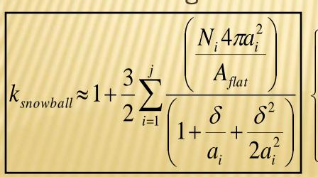
$\begin{cases} a_i = \text{radius of spheres (m)} \\ N_i = \text{number of snowballs of size } a_i \text{ per } A_{flat} \\ A_{flat} = \text{total area containing stacked snowballs} \\ \delta = \text{skin depth (m)} \quad \dots \text{ recall } : \quad \delta = \frac{1}{\sqrt{\pi\mu\sigma f}} \end{cases}$
