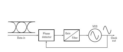
Low frequency jitter is transferred to the clock, high frequency jitter is not
