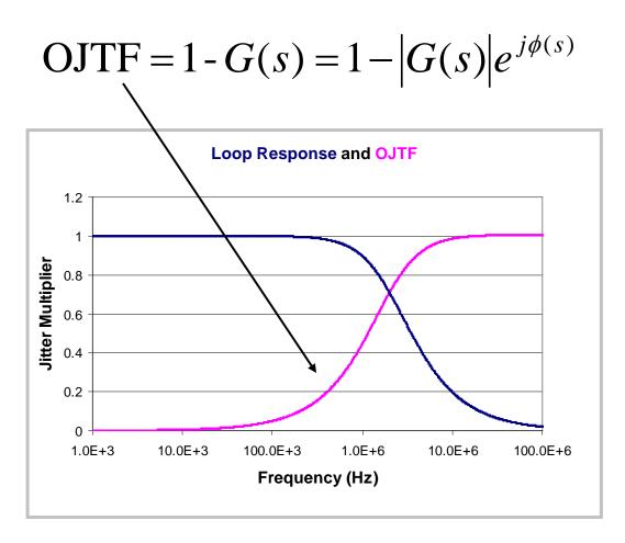
The observed jitter is a complement to the PLL jitter transfer response
