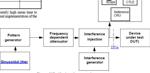
Figure 83D-12—Interference tolerance test setup
