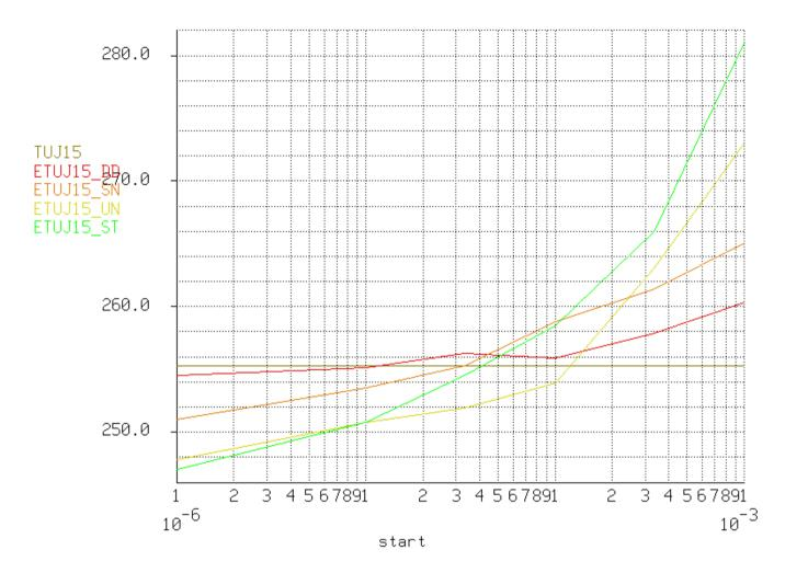
This shows the accuracy of the extrapolated TUJ15 for various cases. It looks like we have a "sweet spot" at start= $10^{-4}$  which is 1/10 the value used in Clause 92. This means that we will need to receive 10x the number of hits which should be OK.
